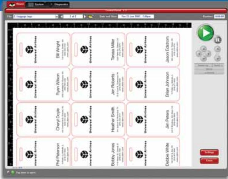
The Laser Interface+ materials-based print driver includes a print preview function which allows users to preview a job on-screen before it is actually run to ensure proper setup. Users can also view and re-run jobs directly from the system at a later time without the need to open the graphic software file.
