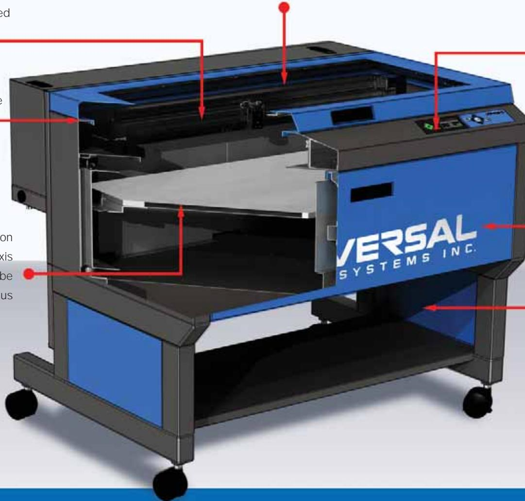
Universal's Professional Series of CO<sub>2</sub> laser systems provide an unbeatable combination of high power (up to 120 watts using dual lasers), three platform sizes and an advanced, materials-based print driver that delivers consistently excellent cutting and engraving results. The Professional Series systems are ideal for high-speed cutting jobs; deep, high-throughput engraving; and fast, permanent marking.
